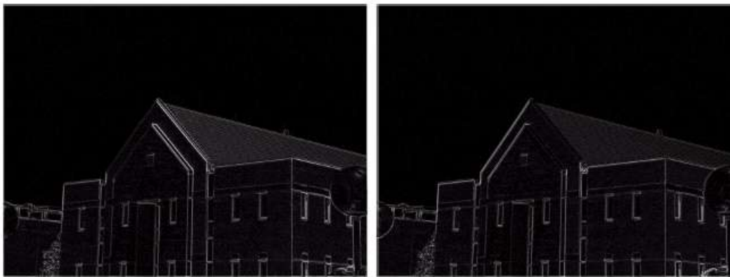
FIGURE 10.12 Diagonal edge detection. (a) Result of using the mask in Fig. 10.9(c). (b) Result of using the mask in Fig. 10.9(d). The input in both cases was Fig. 10.11(a).
